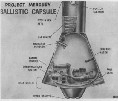
ASTRONAUT'S POSITION inside the Project Mercury space capsule is diagrammed here. "Retro" rockets at the capsule's rear will be fired on signal from the ground or by the astronaut to direct the vehicle's re-entry into the earth's atmosphere. Sandians are helping test the landing system at Salton Sea Test Base.
